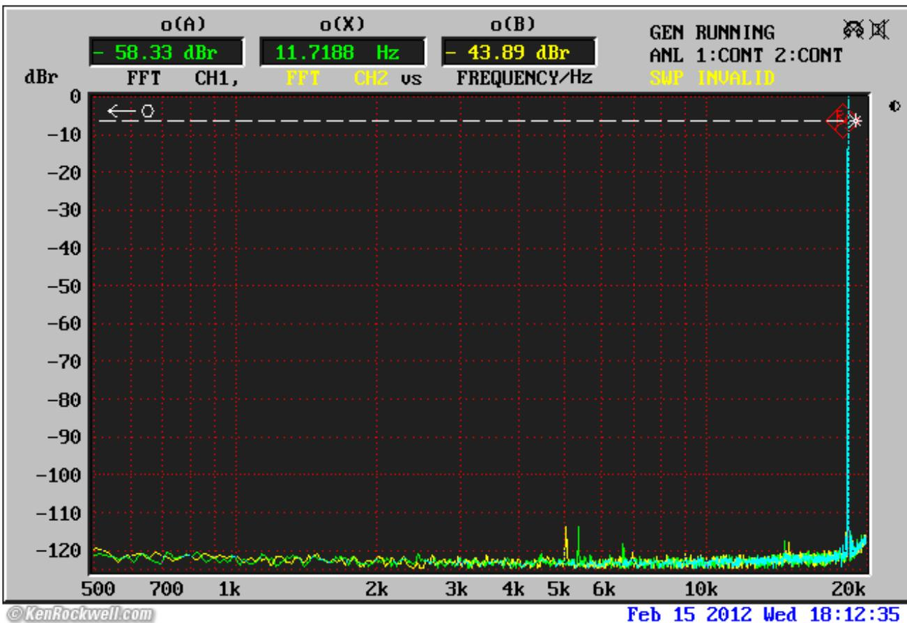
Output spectrum, 20 kHz FS sine, 24-bit 44.1 ksps, with 0.1 UI of jitter at 19 kHz. ([R&S UPL.](#))
