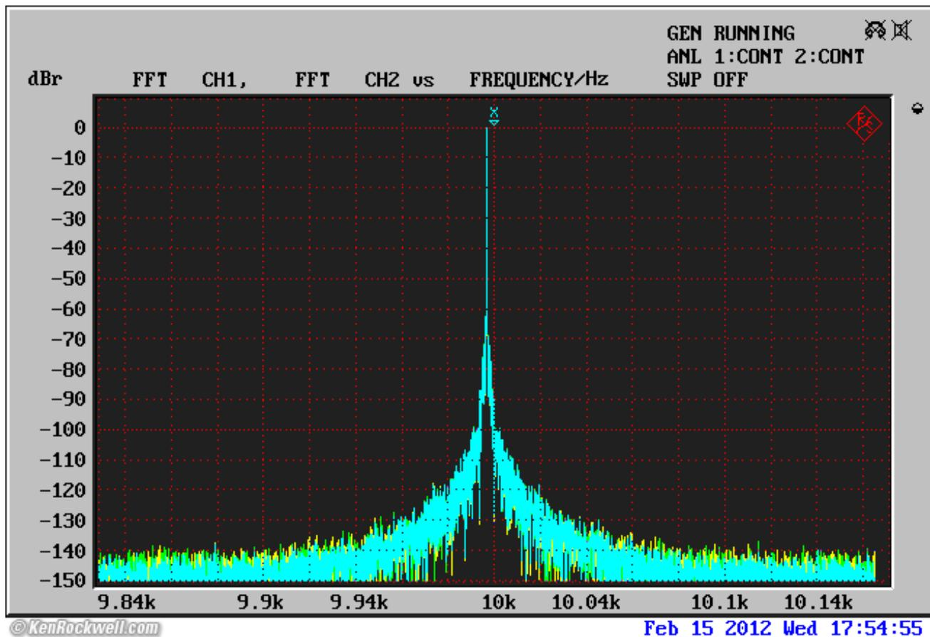
**TOSLINK input, 10 kHz at 0 dBFS 44.1k/24-bits, 2 V RMS line output.**
