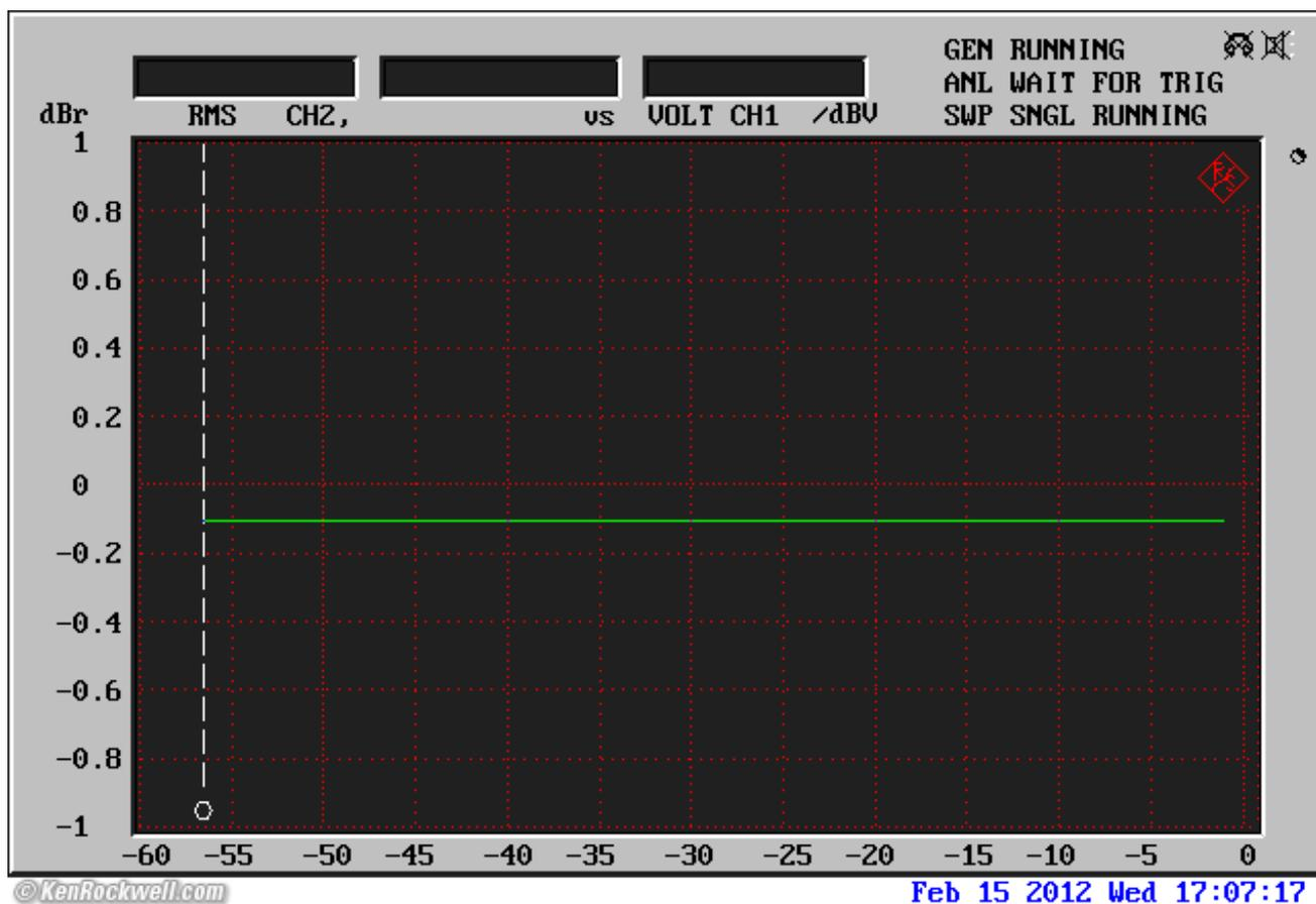
**Right channel level versus left channel volume control setting.** (positive means the image moves to the right. [R&S UPL.](#))
