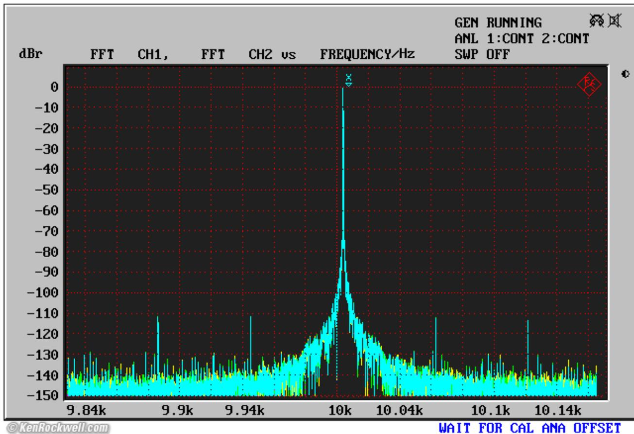
USB input, CBS CD-1 track 9 (10 kHz at 0 dBFS), ALC file played from a 2010 Mac Pro via iTunes, 2 V RMS line output.
