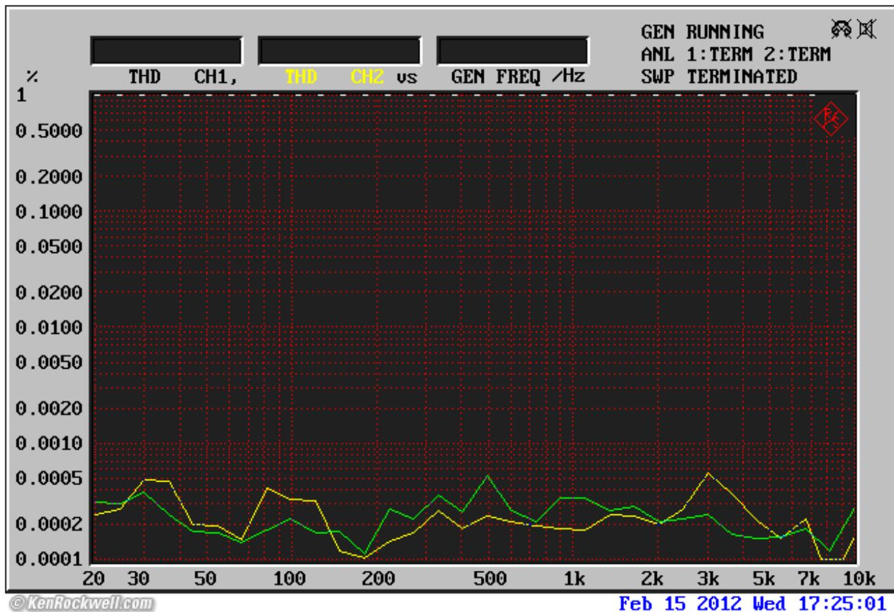
**THD with level control set to maximum, -20 dBFS undithered 24-bit/44.1 input, 200mV output, 22 kHz bandwidth. ([R&S UPL.](#))**
