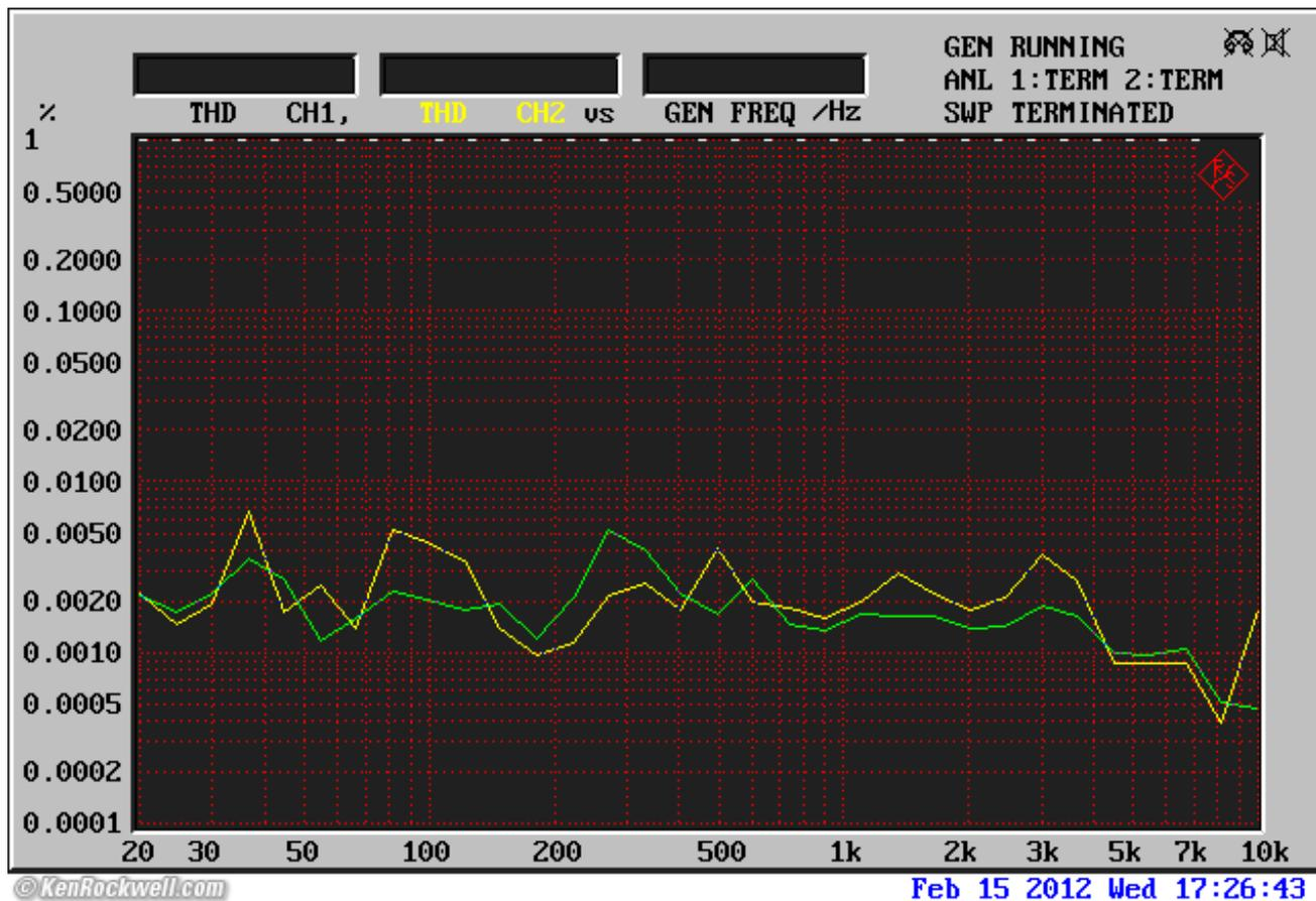
**THD with level control set to maximum, -40 dBFS undithered 24-bit/44.1 input, 20mV output, 22 kHz bandwidth. ([R&S UPL.](#))**
