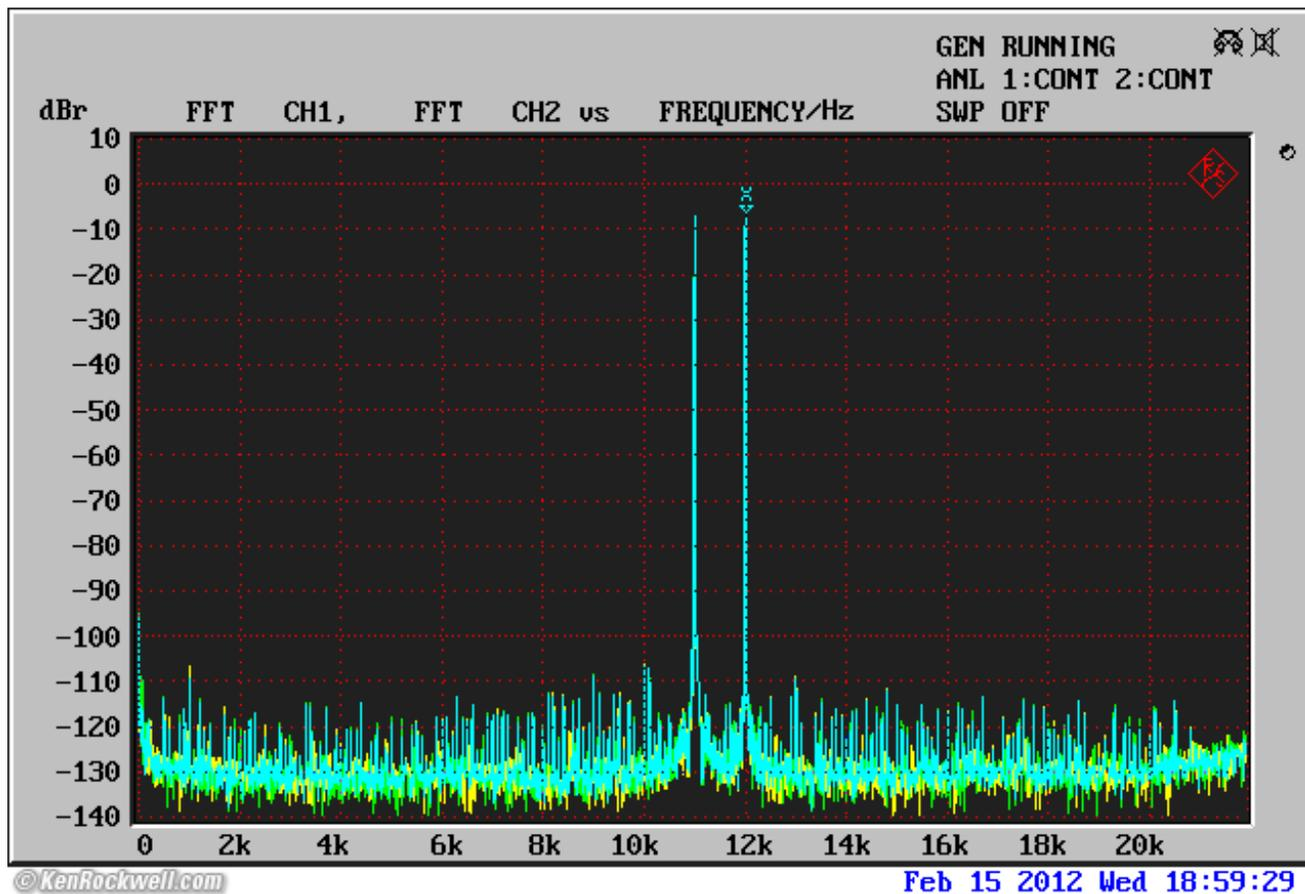
**USB input: audioengine D2 line output at 11 kHz and 12 kHz 1:1. (CBS CD-1 track 13, index 2, [R&S UPL.](#))**
