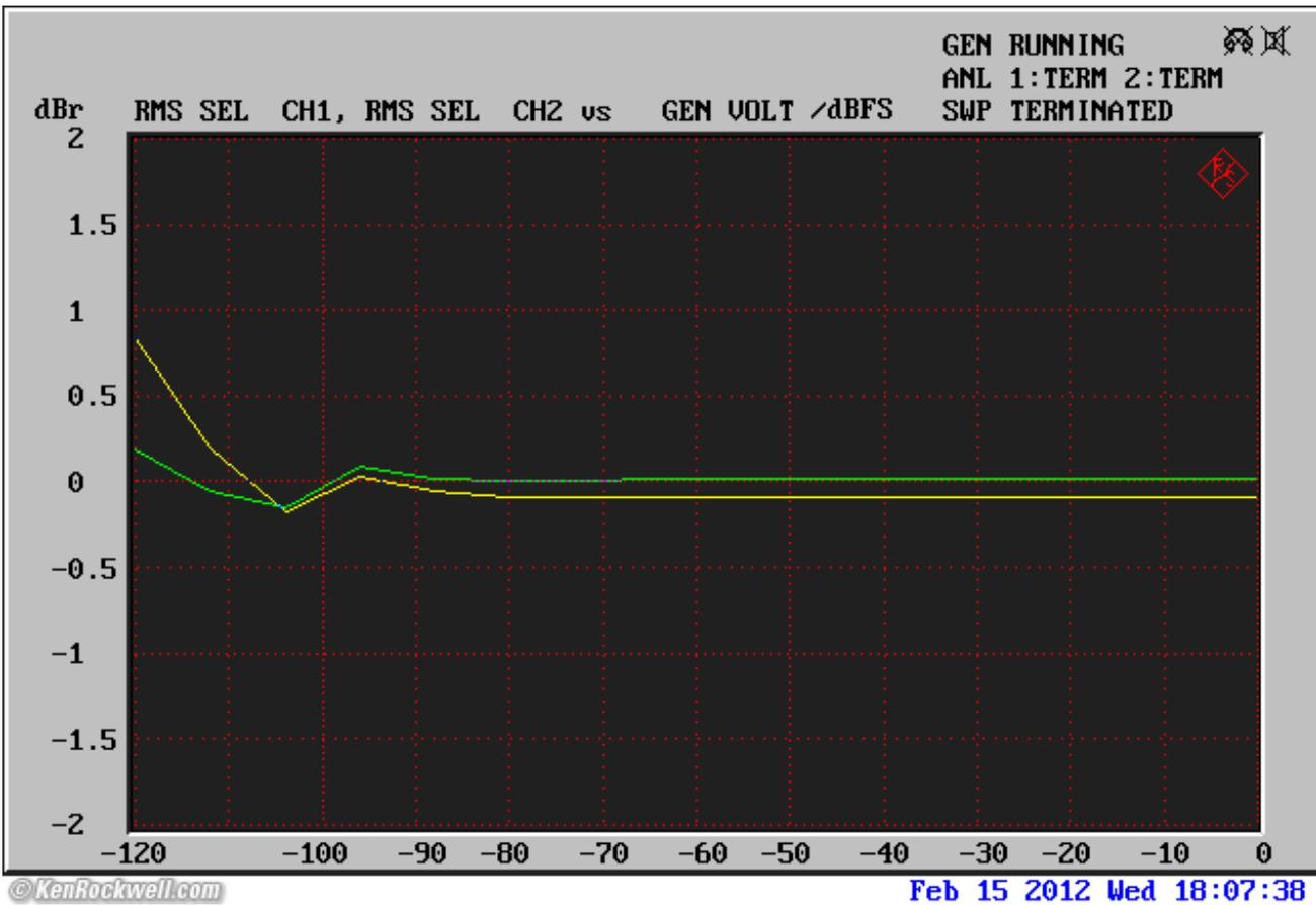
**Level error versus level (linearity), 1 kHz sine, 24-bit 44.1 ksps. ([R&S UPL.](#))**
