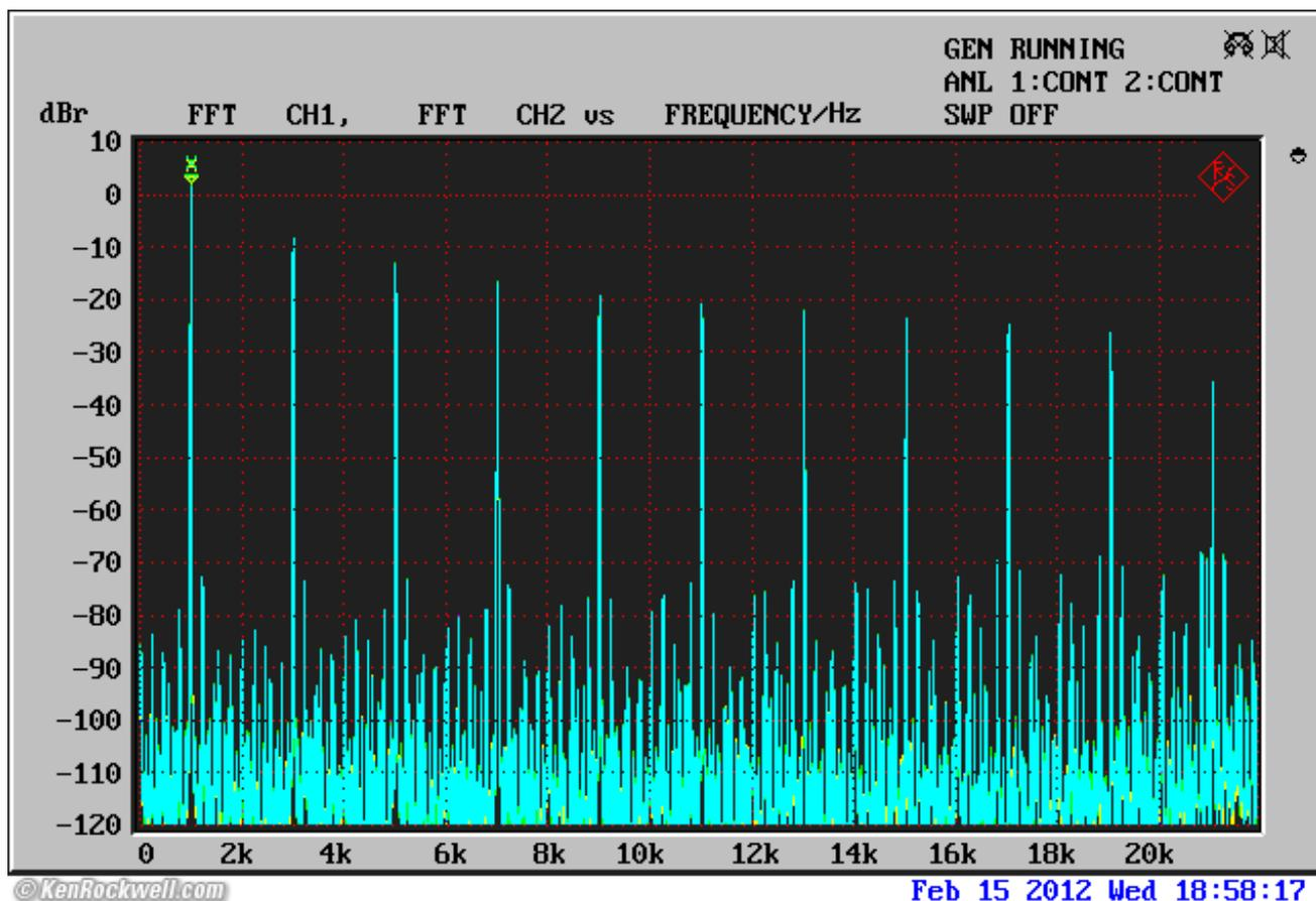
audioengine D2 line output spectrum, 1 kHz square-wave. (CBS CD-1 track 16, [R&S UPL.](#))
