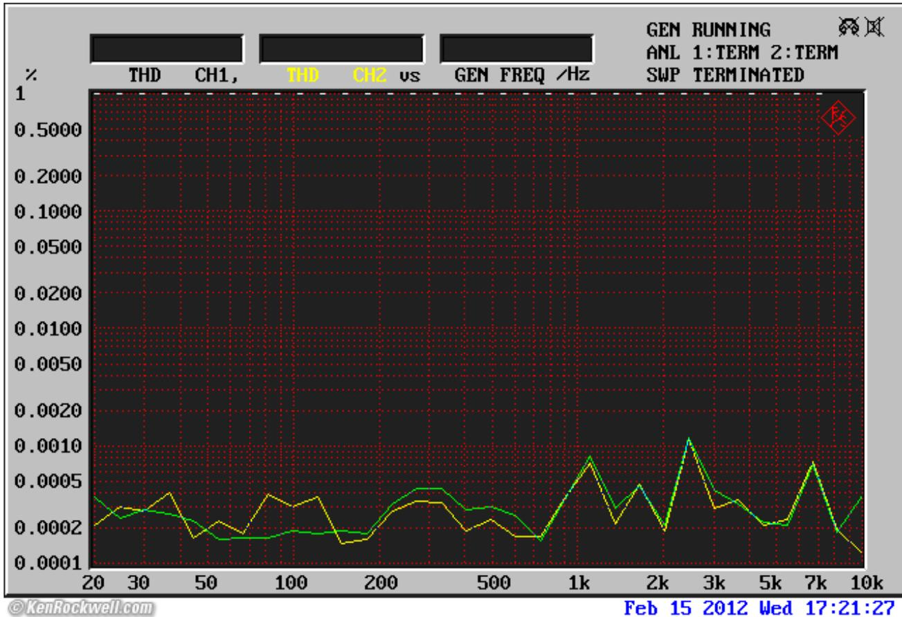
**THD with level control set to -20 dB, 0 dBFS 24-bit/44.1 input, 200mV output, 22 kHz bandwidth. (R&S UPL.)**
