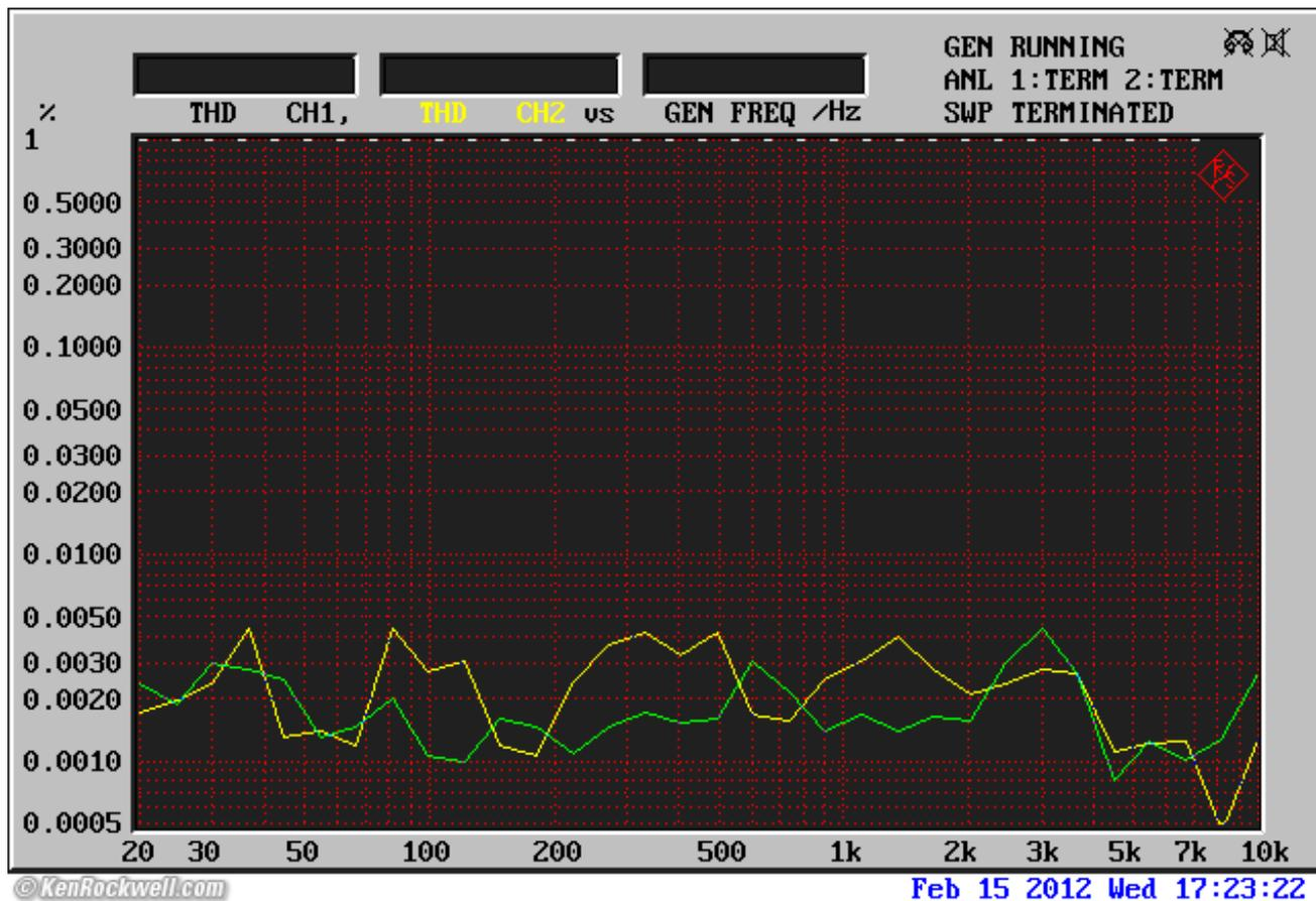
**THD with level control set to -40 dB, 0 dBFS 24-bit/44.1 input, 20mV output, 22 kHz bandwidth. ([R&S UPL.](#))**
