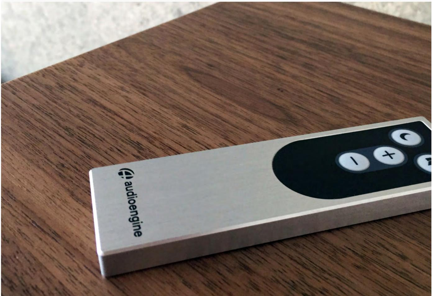
One minor but appreciated detail is the inclusion of a milled aluminum remote that controls volume and playback. Often times, this is a detail that is overlooked and comes packaged in a last-second plastic casing. The remote doesn't add a high-level of functionality, as most users will control volume via a streaming device or universal remote.
