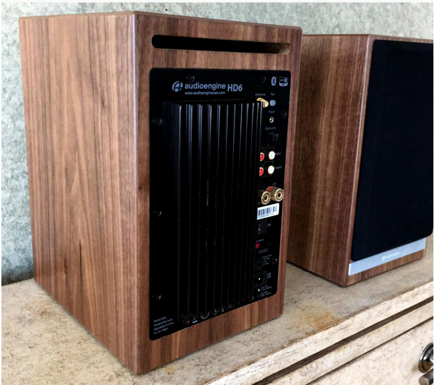
On the backside, you'll find RCA, 3.5mm and optical inputs alongside controls for Bluetooth radio. There is a screw-on antenna near the top of the speaker for those that
