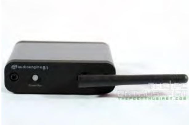
You cannot retract the antenna and it is also not removable. But the antenna can be tilted horizontally to the left or to the right.
