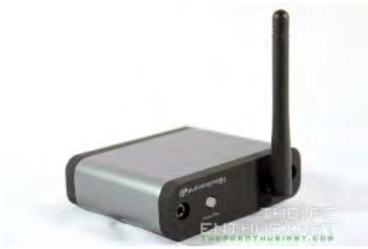
The B1 features a nice, simple and clean design. Its housing is made of aluminum giving it that premium look and feel. It's very sturdy and solid, and it doesn't easily break in case you accidentally dropped it. In front of the B1 are its antenna and a tiny power/pair LED indicator.
