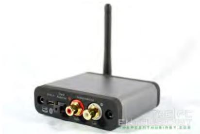
On the back of the Audioengine B1 you will see a 5V DC in micro USB port, an Optical Audio Output port, and an RCA analog output port. I just wish Audioengine also threw in a Toslink cable together with the package, aside from the RCA cable.
