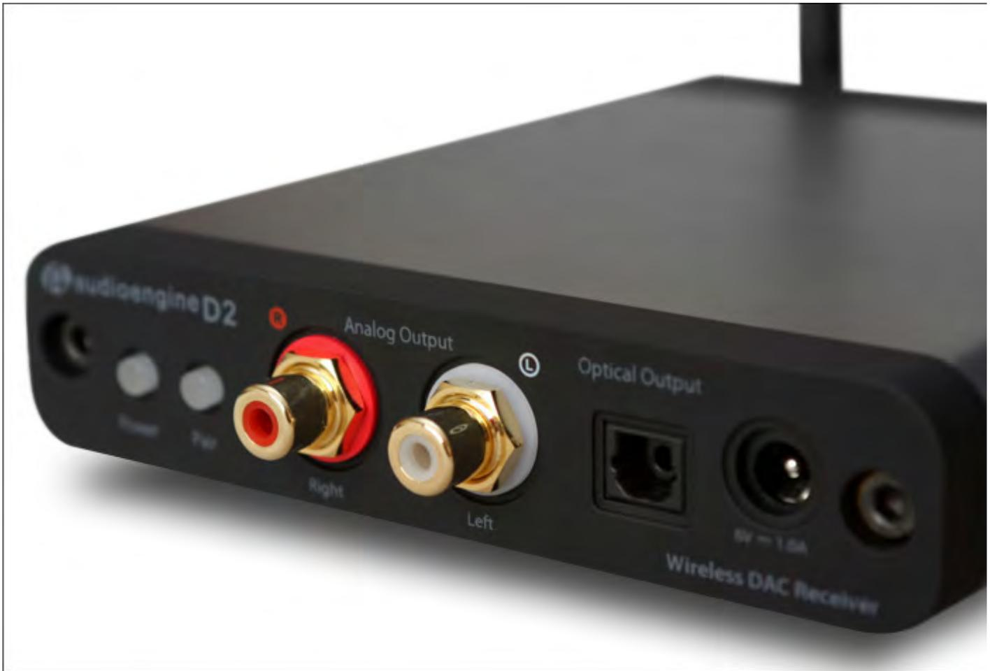
The Receiver has its own Power and Pair lights, an optical digital output for connection to an external DAC, a jack for the wall-wart power supply, and a pair of single-ended RCA jacks for the outgoing analog signal. Most people will probably connect the D2 to an integrated amplifier or preamplifier, but the fact that it has its own volume control makes it possible to be directly hooked up to a power amp or active speakers.
