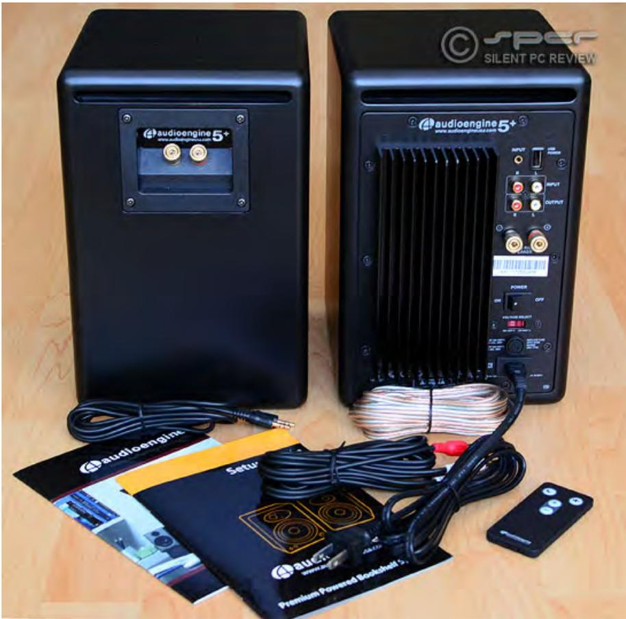
*The rear view of the satin black finish A5+, plus the other contents of the package: mini-jack audio cable, 2m; RCA to RCA audio cable, 2m; 16AWG speaker wire, 3.75m; detachable power cord; setup guide. Note the slot vent across the top portion of each speaker's back panel.*
