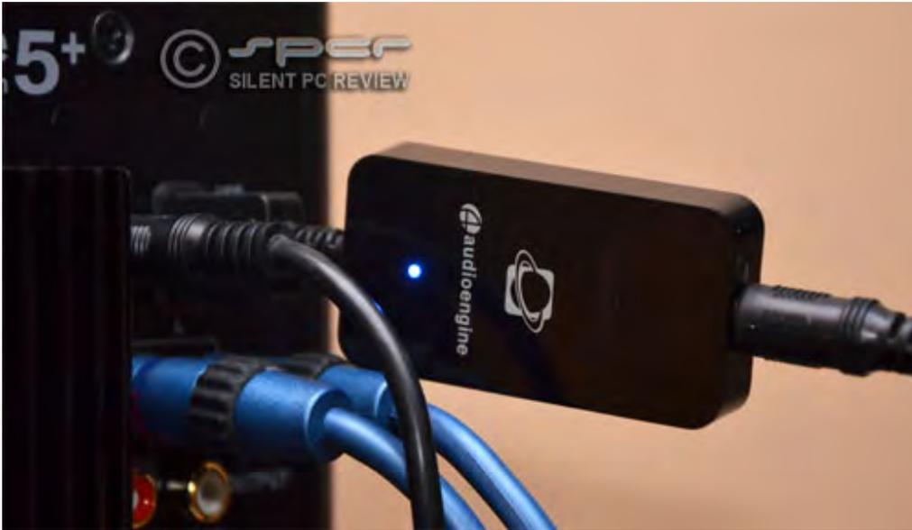
*W1 receiver powered by USB port on A5+ speaker, with mini-plug lead from it into the mini-input on A5+. The RCA phono jacks were unplugged before testing.*
