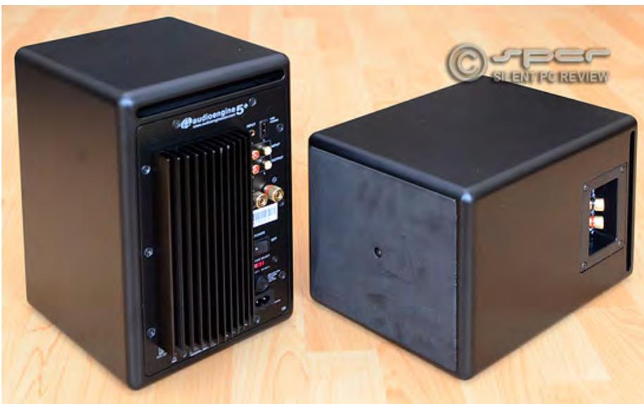
*The rounded-corner enclosures are made of MDF and have a nice solid heft and feel, with a good satin black finish. A dense cushioned pad is fixed to the bottom panel, which also has a 1/4" threaded insert for stand mounting. A stand with such hardware is not offered at the Audioengine web store at this time,*
