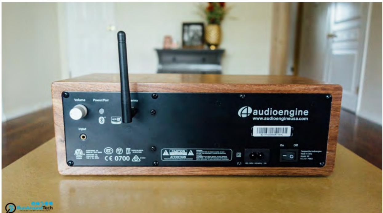
The back of the B2 features controls for the volume, inputs, power, and Bluetooth connectivity. The B2 connects via a 3.5mm cable or Bluetooth only. The volume knob is easy to reach from the front of the B2, and even it oozes of quality. The Bluetooth connectivity range is greatly increased thanks to an included antenna that screws into the connector on the back.
