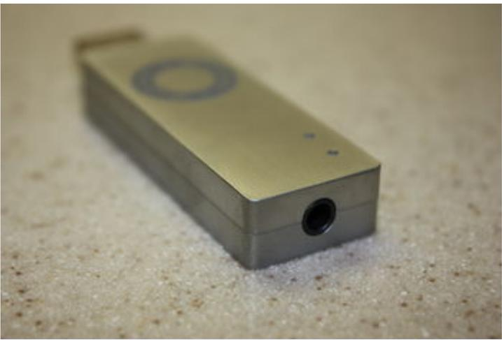
Here we see the top and bottom. The unit has a very minimalistic design. The logo and two white and blue LEDs are the only accents to the silver. The white LED illuminates when power is present and the blue LED illuminates when the audio signal is HD or above 48kHz. This blue LED will let you know you are getting the most out of your DAC.
