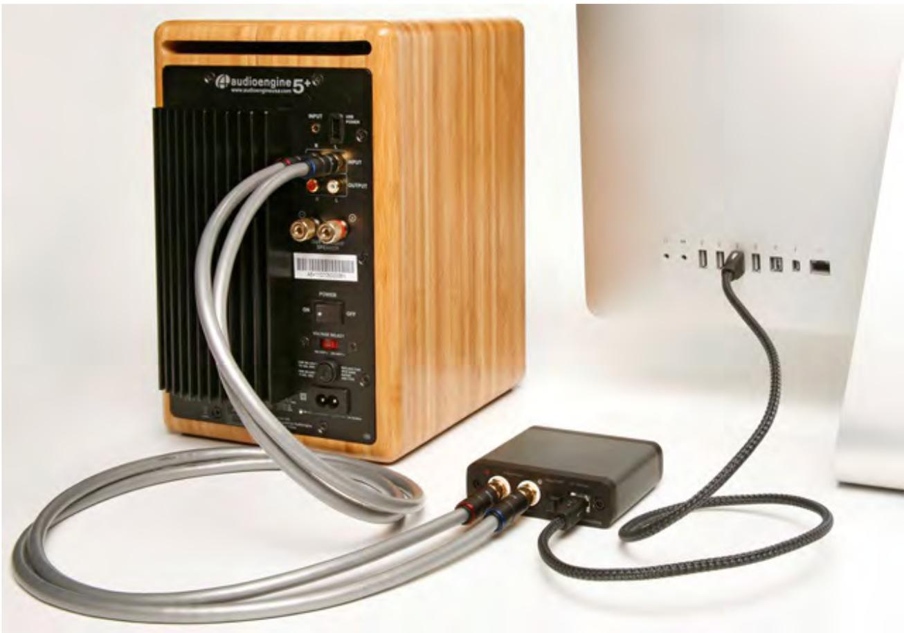
Installation couldn't be easier. A simple USB powered connection from the iMac into the D1, then a RCA cable pair into the A5+'s, and you're off to the races. No drivers needed. I tested this on my Windows 7 laptop and the experience was the same, but this device was bound for my home setup. And a tip for the Mac users out there, you should dive into the built-in MIDI setup and set the D1 as your output, and set it to 24-bit mode.
