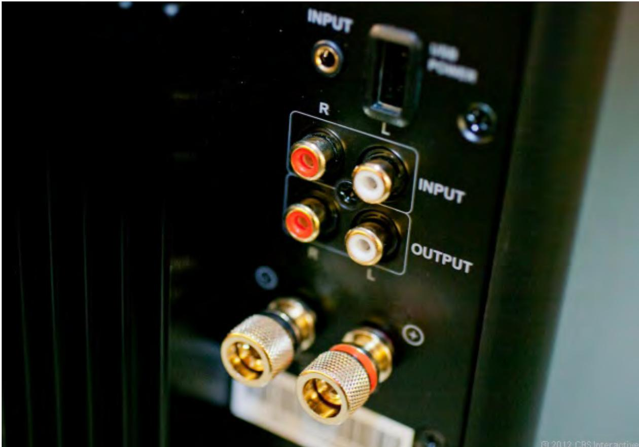
**You get two inputs, a subwoofer output, a USB power port, and speaker wire connections to link to the other speaker.**
