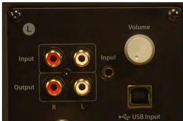
There are a number of inputs on the Audioengine 2+ including USB, 3.5mm, and an RCA analogue input. Analogue outputs are included for integrating with a sub for additional bass. There is no crossover in the 2+ speakers though Audioengine says they have integrated a limiter to stop distortion. In our tests, we found that low bass sweeps would produce some port chuffing and flutter but in actual playback it wasn't much of an issue.
